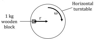
a) The student wants to use this equipment to investigate how the radius of the wooden block's circular path (r) affects the angular velocity of the turntable when the block slides off.
