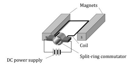
Which component changes the direction of the current in the motor?
