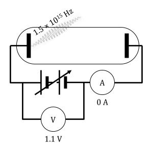
The voltage across the glass tube was increased to 1.1 V, at which point the photocurrent stopped flowing.
