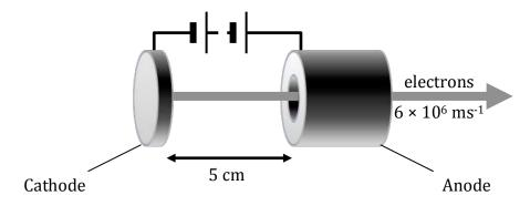
The electron gun accelerates an electron from rest to a velocity of  $6 \times 10^6$  ms<sup>-1</sup>.
