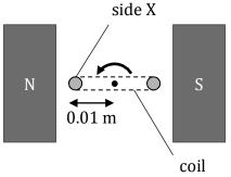
The coil has an area of 1  $\times$  10  $^{\!\!\!-3}$   $m^2.$  The torque on the coil in the position shown is 0.03 Nm  $^{\!\!\!-1}.$
