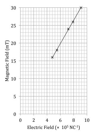
$$qE = qvB : v = \frac{E}{B} = \frac{1}{\text{gradient}} = \frac{1}{3.3 \times 10^{-8}} = 3.0 \times 10^7 \text{ ms}^{-1}$$
