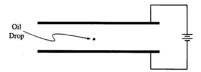
Suppose that when the potential difference between the plates is adjusted until the electric field is  $10~000~NC^{-1}$  downward, a certain drop with a mass of  $3.27 \times 10^{-16}$  kg remains suspended.
