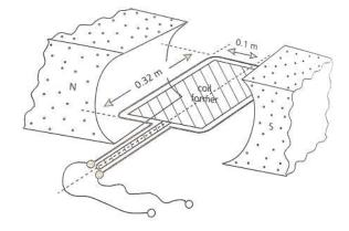
An electric motor consists of a 100-turn coil of wire on a frame that is free to rotate in a radial field as shown in the figure above. The field strength is 25.0 mT and the coil dimensions are 0.32 m in length and 0.1 m wide. The effective voltage driving the motor is 120 V DC.
