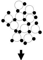
PARTICLE VIEW AFTER COMPLETE BOILING
