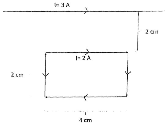
Consider the situation shown in the diagram above where a wire carrying a current of 3 A is placed near a rigid rectangular loop carrying a current of 2 A (clockwise). Calculate the net force acting on the wire loop. (You may consider the wire to be parallel to the long side of the rectangle.)
