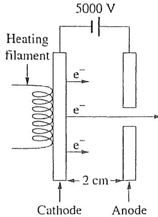
Electrons leave the cathode and are accelerated towards the anode. (The electric field between the cathode and anode can be considered uniform.)
