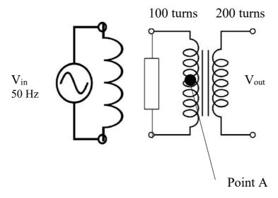
Using the information in the diagram, and assuming ideal conditions, calculate Vout.
