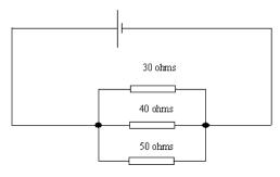
The current through the 50 ohm resistor is closest to
