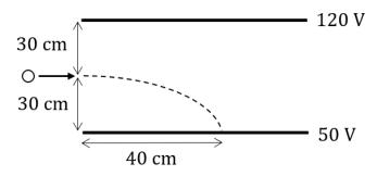
Using the motion of the charged particle, what can be concluded about the charge of the particle and the work done by the electric field?
