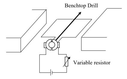
The variable resistor is adjusted to have a large resistance when the motor is starting up and the resistance is slowly lowered as the motor reaches its operating speed.
