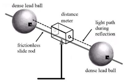
Lucy rotated the apparatus creating a centripetal force. The aim was to find the speed at which the centripetal force was equal to the gravitational force between the two dense lead balls.
