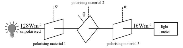
If the intensity of the light passing out of the third filter is 16 Wm<sup>-2</sup>, calculate the angle ( $\theta$ ) with which the polarising material 2 is rotated?
